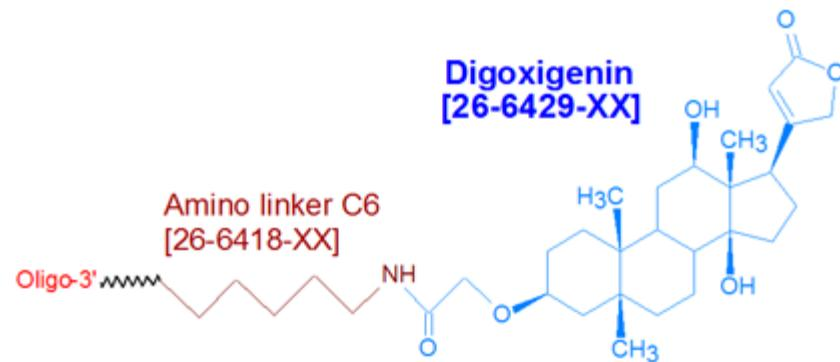
This modification is a post synthesis conjugation to a primary amino group thus an additional modification with an amino group is required. A C3, C6 or C12 amino group can be placed at the 5' or for the 3' end a C3 or C7 amino and for internal positions an amino modified base is used, e.g Amino dT C6.
