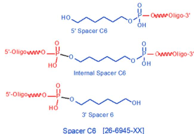
Spacer modifications C2, C3, C4, C6, C9, C12 and triethylene glycol Spacer 9 and 18 are used to insert a spacer arm in an oligonucleotide. These modifications can be added in multiple additions when a longer spacer is required. 3'-Spacer C3 CPG may also act as a blocker of exonuclease and polymerase activity at the 3'-terminus. dSpacer is used to introduce a stable abasic site within an oligonucleotide. See "Photo-Cleavable" modification category for photo-cleavable Spacer.
