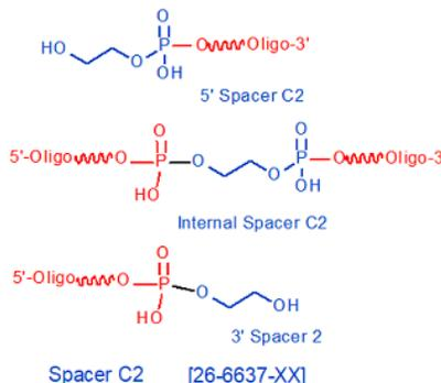
Spacer modifications C2, C3, C4, C6, C9, C12 and triethylene glycol Spacer 9 and 18 are used to insert a spacer arm in an oligonucleotide. These modifications can be added in multiple additions when a longer spacer is required. 3'-Spacer C3 CPG may also act as a blocker of exonuclease and polymerase activity at the 3'-terminus. dSpacer is used to introduce a stable abasic site within an oligonucleotide. See "Photo-Cleavable" modification category for photo-cleavable Spacer.
