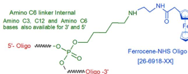
This modification is a post synthesis conjugation to a primary amino group thus an additional modification with an amino group is required. A C3, C6 or C12 amino group can be placed at the 5' or for the 3' end a C3 or C7 amino and for internal positions an amino modified base is used, e.g Amino dT C6.
