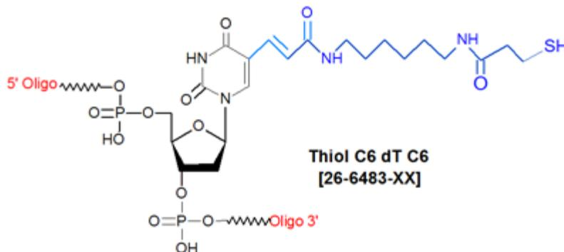
Thiol-C6 dT is a thiol modifier designed to functionalize an oligonucleotide at an internal T position for conjugation to the desired solid support e.g gold. The resulting thiol group is separated from the oligo by a six-carbon spacer arm, to reduce steric interactions with the end of the oligo.
