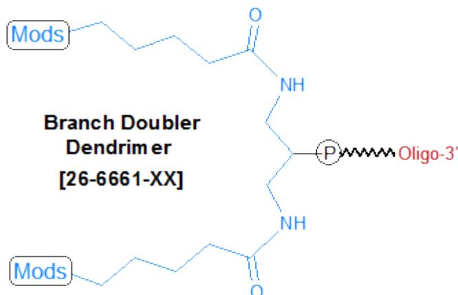
Branch Doubler C2, Branch Doubler C8, Trebler and Long Trebler Dendrimer are oligonucleotide modifications that can be added to synthetic oligos to create branches. Multiple additions of these branching modifications are primarily used to add/conjugate ligands, fluorescent labels, tags and other modifications to increase sensitivity and multiple attachment points.
