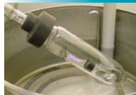
PHOTO 3: VIAL IN ROTARY EVAPORATOR
